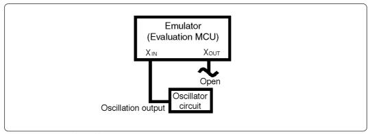
Figure 3.1 External oscillator circuit
